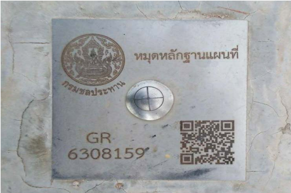
Fig.2 Standard bench mark
