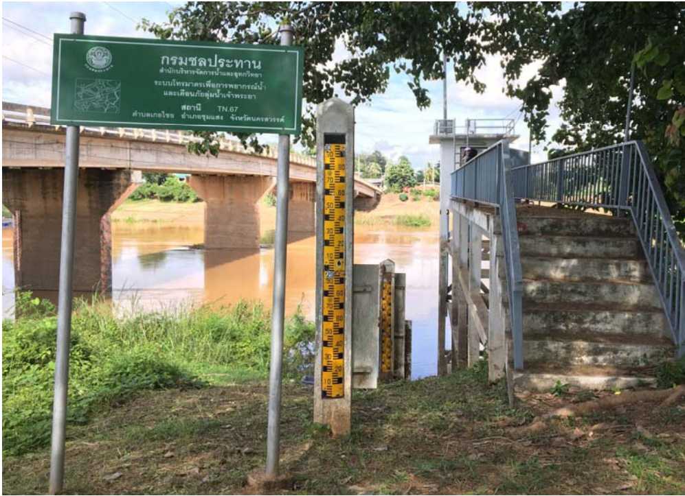
Fig.1 Typical vertical staff gauge
