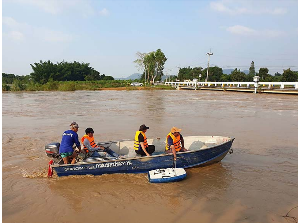
Fig.3 Discharge Measurement by River Surveyor M9 ...etc.
