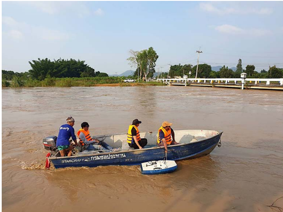
Fig.3 Discharge Measurement by River Surveyor M9 ...etc.
